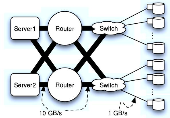
(b) Disks connected to redundant servers. Switch failure is still an issue, but routers allow for more redundancy.
