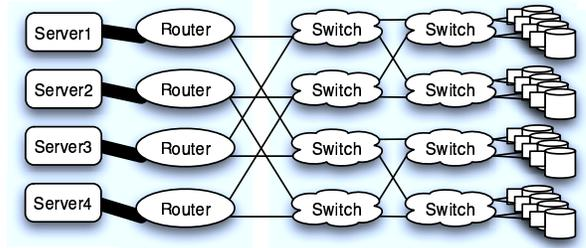
**Figure 3. Disks connected in a butterfly network topology.**
