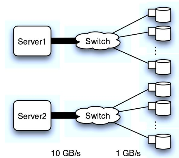
(a) Disks connected to a single server. This configuration is susceptible to loss of availability if a single switch or server fails.
