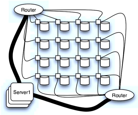
(a) Disks connected in a mesh topology.
