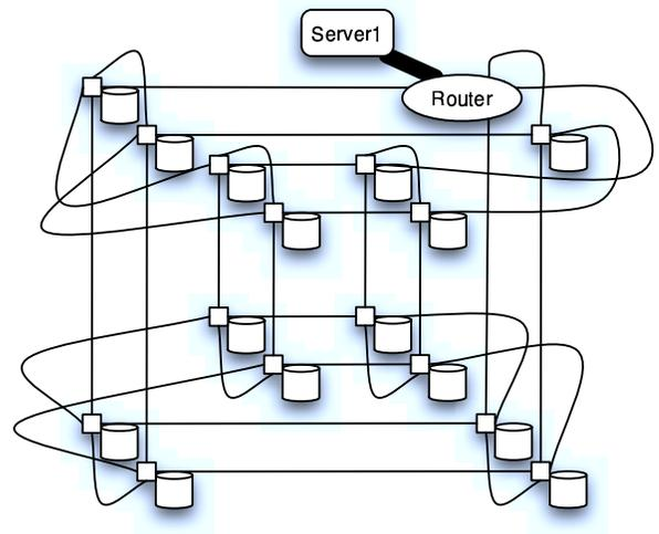
**Figure 5. Disks connected in a hypercube topology.**
