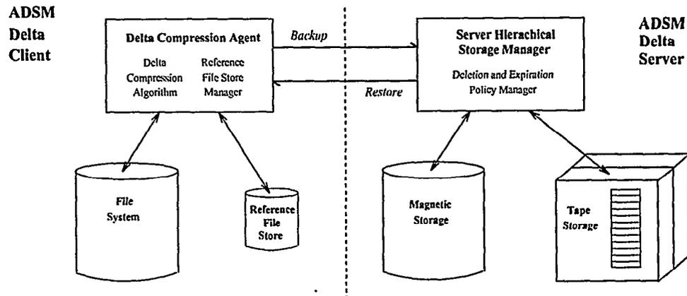
Figure 1: Client/server schematic for a delta backup system.
